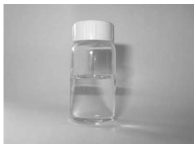
Fig. 6 Polytrimethylene ether glycol formed under optimum conditions, with low color. On larger scale, water is injected at a known addition rate to prevent color formation.
