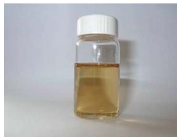
Fig. 1 Polytrimethylene glycol formed at 170 °C, using 1 wt% TFESA, after 7 h.
